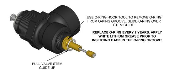
Figure 6G – STEP 6 – Replace valve seat and valve stem base o-rings.
