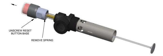
Figure 6C – STEP 3 – Replace button post internal o-ring
